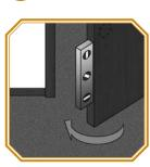
1 Pull door toward you to check if it's level. Observe contact of door to jam and make sure it's level. Adjust if
