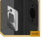
10 For Latch Strikeplate: Insert dustbox into hole, add inserting #8 x 3/4" wood screws into pilot holes.
