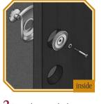
2 Insert dummy cylinder through dummy cylinder collar and into outside of door. From inside, insert retaining screw through lock washer and locating plate, then scre into dummy cylinder.
