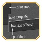
2 (Aerial View) To ensure proper alignment, only use hole template on side facing **Helpful Hint:** Some doors have a beveled edge with bevel facing doorstop.
