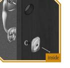
inserting the #10-32 x  $2\frac{3}{4}$ " oval head screw on inside of door through rectangular screw base and the lower hole (C). Leave **Note:** Go to door preparation if you do not have a lower
