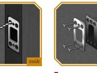
7 For Deadbolt Strikeplate: Insert dustbox into hole, add reinforcing strike, and secure with four #8 x <sup>3</sup>/<sub>4</sub>" combination screws. Two screws are supplied with active trim and two are supplied with dummy trim.
