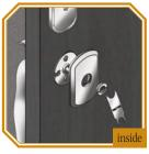
inside adapter. Using rose retainer wrench, thread the rose retainer onto the threaded portion of the adapter.
