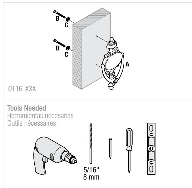
**1** Center template on EXTERIOR side of door. Ensure template is level, and mark holes.
