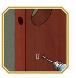
8 Very carefully drill (E) <sup>5</sup>/<sub>16</sub>" hole into door exactly at pencil mark.
