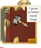
**10** From inside of door, insert short end of spindle through the latch with the V groove on the long end angled down and toward hinges. Position outside handleset trim so spindle slides into square hole in thumbpiece cartridge **Note:** Make certain spino is inserted through the latch to stops.
