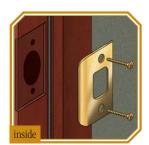
9 For Latch Strikeplate Insert dustbox into hole, add strikeplate, and secure by inserting #8 x <sup>3</sup>/<sub>4</sub>" wood screws into pilot holes.
