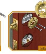
**6** Place turnpiece mounting plate on inside of door. Attach to cylinder using two #10-32 x 1<sup>7</sup>/<sub>8</sub>" pan head screws. Tighten screws. Important: Note orientation of mounting plate.
