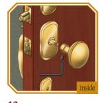
13 Slide knob onto spindle and tighten set screw with Allen wrench. Knob/lever is secured when set screw enters V groove in spindle.
