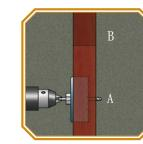
5 Very carefully drill (A, B) 21/8" holes into one side of door face until drill bit starts to protrude on opposite side. Important: Drill perpendicularly (at a 90° angle) to door.
