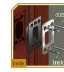
6 For Deadbolt Strikeplate: Insert dustbox into hole, add reinforcing strike, and secure with 3" reinforcing screws (outside holes) and #8 x <sup>3</sup>/<sub>4</sub>" combination screws (inside
