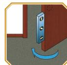
Pull door toward you to check if it's level. Observe contact of door to jam and make sure it's level. Adjust if necessarv
