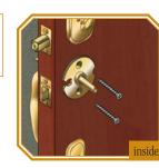
**11** Align spindle, latch, and outside handle. Insert the inside adapter onto the posts of the outside handleset trim. Secure with two  $\#10-32 \ge 1\frac{1}{4}$ flat head screws. Tighten all three screws, including screw for bottom of handle.
