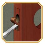
**10** Chisel faceplate cavity <sup>5</sup>/<sub>22</sub>" deen Helpful Hint: Chisel toward inside edge of score lines, removing only a small bit to avoid wood damage.
