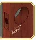
Determine your backset, which is the distance from the edge of door to center of hole. Your lockset is shipped with a 2<sup>3</sup>/<sub>8</sub>" backset (most common). Adjust for a  $2\frac{3}{4}$ backset door only.
