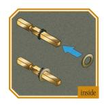
9 Measure the thickness of your door. If door is less than 1<sup>3</sup>/<sub>4</sub>" thick, do not use the spacer provided. If your door measures 1<sup>3</sup>/<sub>4</sub>", slide the spacer onto spindle.
