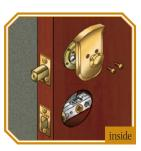
Place inside turnpiece over mounting plate. Insert tailpiece into inside turnpiece. Attach inside turnpiece to mounting plate with two #8-32 x 3/4" oval head screws. Make certain turn knob rotates smoothly in both directions.
