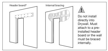
\*Header board and anchor screws not included.
