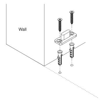
Tip: Install floor guide in a position where it won't be exposed with door in the open or closed position.
