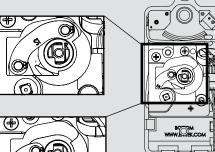
Cam link must remain in the correct position during installation.
