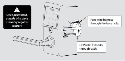
With the Outside Trim Plate Assembly flush to the door, **REMOVE** the Plastic Extender.
