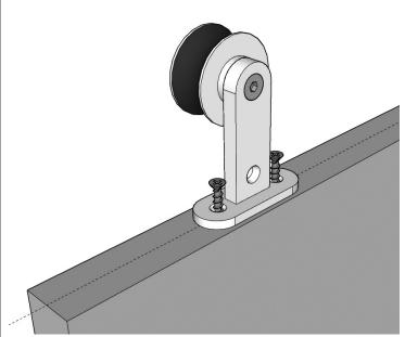
Determine your Door Roller Hardware position. Measure and mark the center line on top of the door. Position each roller on top of the door a minimum of 2" from the edge or center of the stile. Install with (4) Door Roller Hardware Screws.
