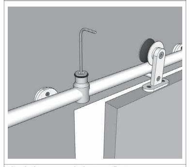
Adjust the door stops accordingly using an Allen Key.
