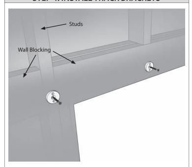
When installing into the solid wood block or wall, insert using the provided wall screws. Align each track bracket level on the center line mark and install with (6) bracket screws.
