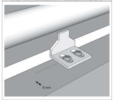
After door stops are adjusted, measure and mark 8 mm from the back on top of the door. Position the Soft-close Brackets to engage the Soft-close guide when it opens and closes. Mount and adjust the Soft-close Brackets using the screws provided.
