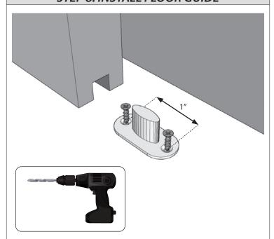
Once the door is plumb, position the floor-mounted door guide inside the mortised door, line up close to the opening. Slide the door side-to-side to ensure functionality for final placement then mark holes with a pencil and predrll 1/4" holes. If drilling directly into concrete floor, use the provided anchors.
