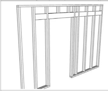
**NEW CONSTRUCTION:** Wood blocking can be installed inside the wall in a new construction.
