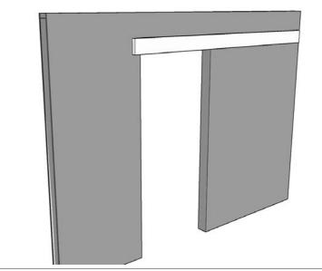
**SURFACE MOUNTED:** The track can be installed using surface wood blocking mounted to the structural surface of a wall using mounting screws into studs. Use a stud finder where necessary to locate studs and safely secure.
