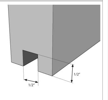
Mortise a 1/2" wide x 1/2" deep groove in the center bottom of the door to use with the floor-mounted door guide. This will prevent the door from swinging in and out and ensure smooth travel side-to-side.
