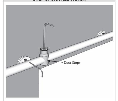
Determine where your Door Stops needs to be placed prior to mounting. Insert one Door Stop on each side of the track inside the first mounting hole before securing if needed.
