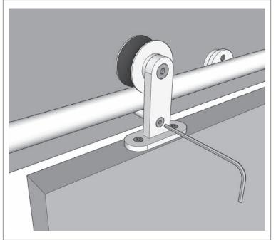
Mount Anti-jump Rods into position using an Allen Key.
