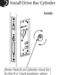
fully screwed into lock body.
