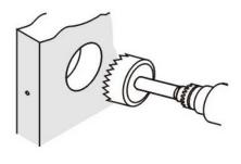
Drill 1" (25mm) hole in center of door edge through to 2-1/8" (54mm) hole for latch. Check template for correct size for your latch application.
