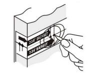
Mark center hole on door face through guide on template for either 2-3/8" (60mm) or 2-3/4" (70mm) backset.
